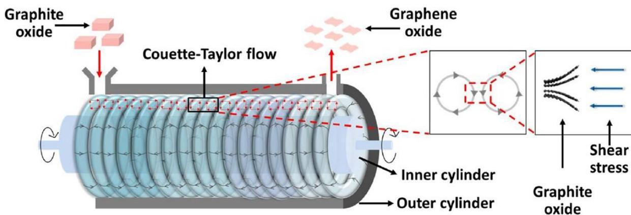
**Fig 4.** Conceptual illustration of Taylor-Couette Flow method of graphite oxide exfoliation via shearing stress. (Park et al., 2017)
