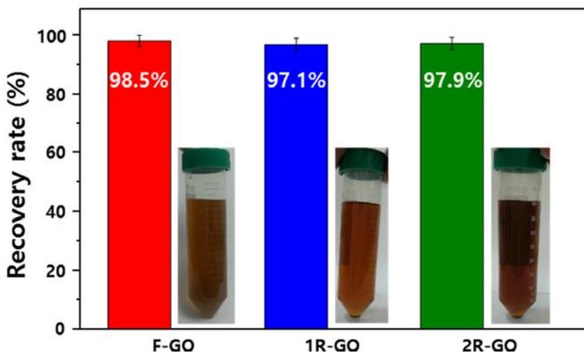
**Fig 6.** Recovery rate of the graphene oxide obtained with fresh (F-GO), once-recycled (1R-GO), and twice-recycled (2R-GO) sulfuric acid. (Park et al., 2017)
