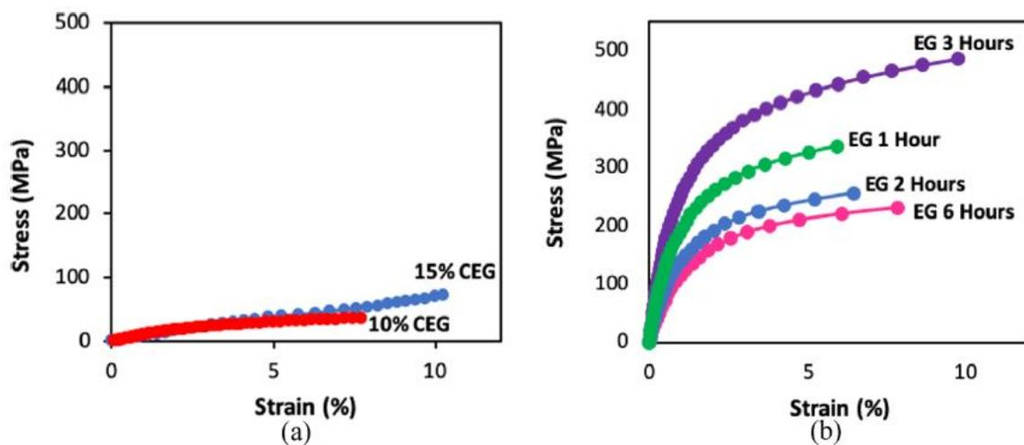
**Fig 5.** Mechanical properties of graphene fibers. (a) commercially available expandable graphite (CEG) and (b) expandable graphite from Taylor-Couette method. (AlAmer et al. 2020)
