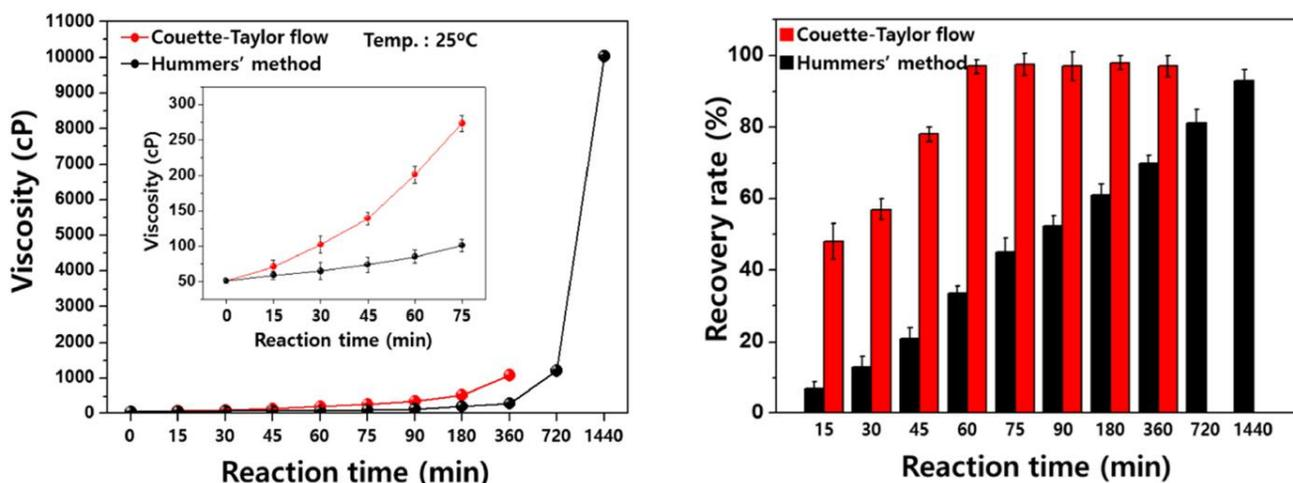
**Figure 1.** Comparison of the Hummer’s Method and Taylor-Couette Flow Method. (Left) Viscosity of the graphite oxide mixture with varying reaction times. (Right) Recovery rate of GO in accordance with the reaction time. (Park et al., 2017)
