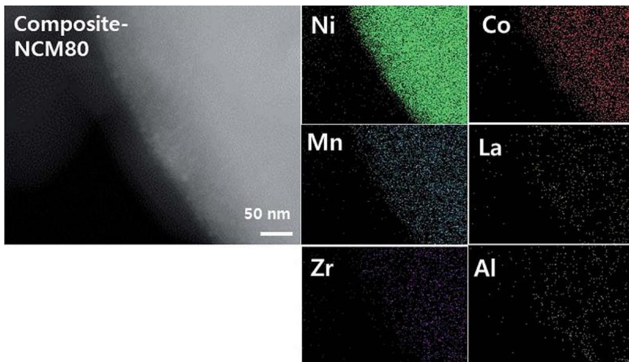
EDS mapping images display uniform distribution of Ni, Co, Mn, La, Zr, Al on coating of composite NCM-LZAOH material synthesized in Taylor-Couette Reactor
