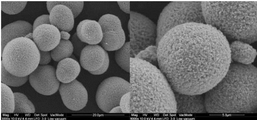
SEM images from Argonne National Laboratory's synthesis of NCM811 with the Taylor Vortex Reactor
