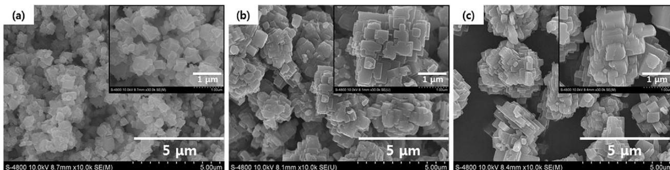
SEM images of Na-ion battery materials synthesized in the Taylor Crystallizer at various temperatures. (a) 25°C and air-dried, (b) 60°C and air-dried, (c) 60°C and vacuum-dried
