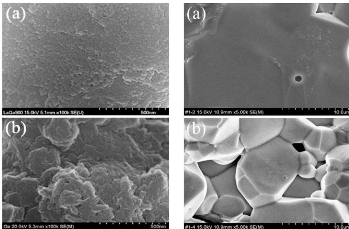
Left: SEM Image of Ga-doped LLZO precursor synthesized in (a) Taylor Crystallizer and (b) Batch Reactor
