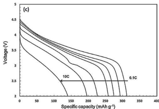
Electrochemical performance of Mn-rich NMC battery precursors and cathode materials synthesized in Taylor Vortex Reactor.
