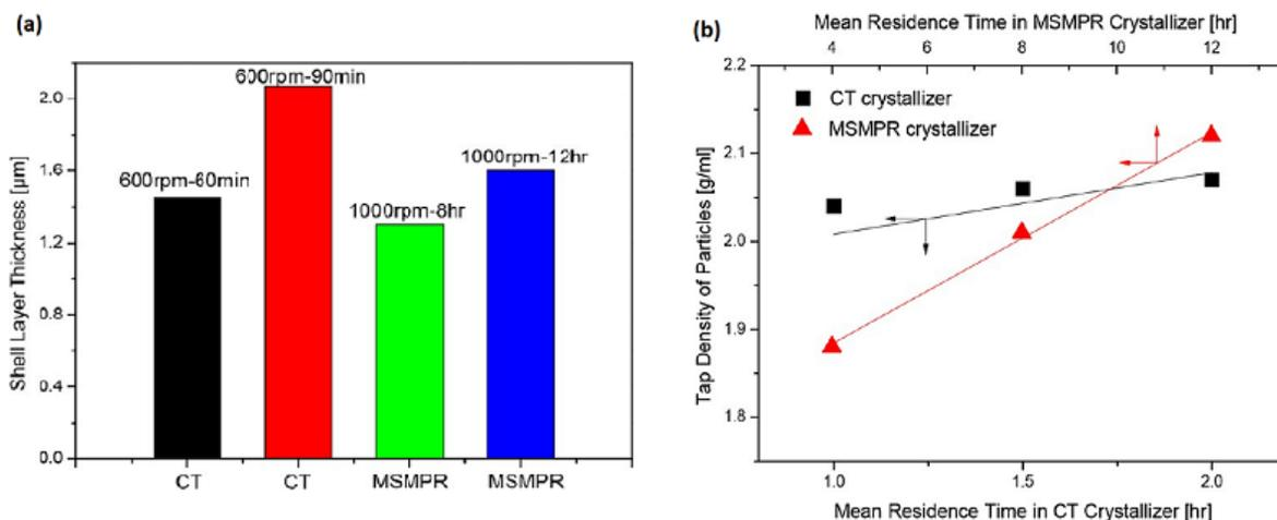
NMC Core-Shell Crystallization in a Taylor-Couette Reactor vs. MSMRP (a) Shell Layer Thickness vs. Mean Residence Time, (b) Tap Density vs. Mean Residence Time.
