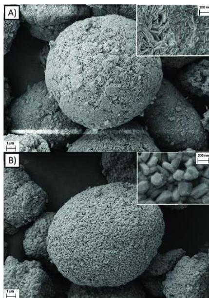
SEM images of (A) NMC Precursor Material produced by Taylor Vortex Reactor and (B) Lithiated NMC Material
