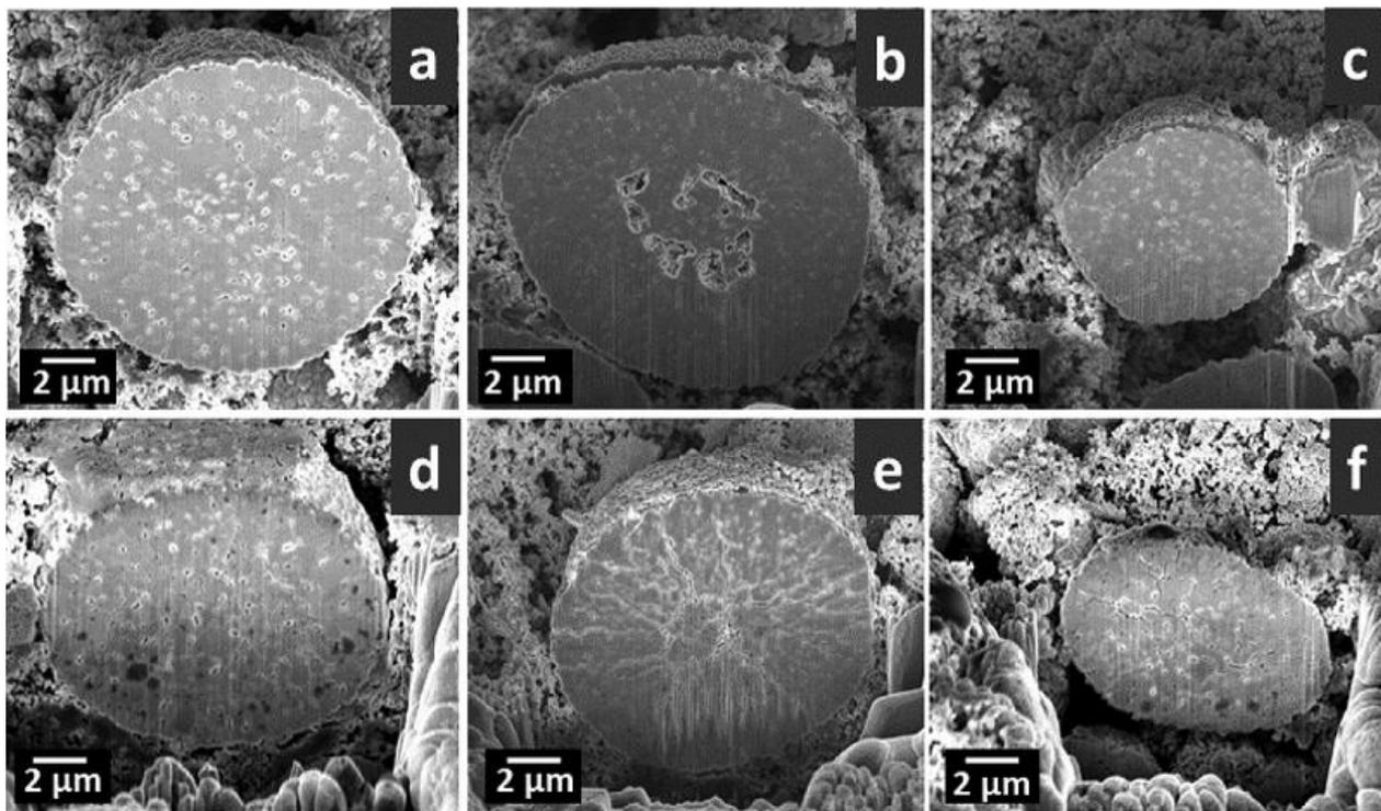
SEM Images of pristine and cycled (a, d) LNO, (b, e) LNMO, and (c, f) LNCO cathode particles synthesized in Taylor Crystallizer.
