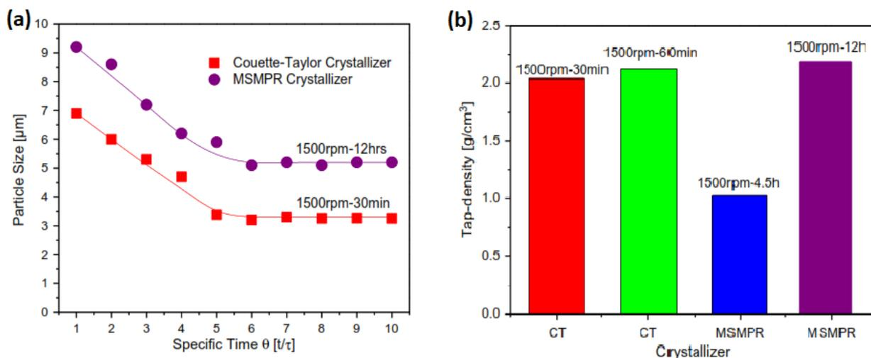
Comparison of Ni-rich hydroxide production between Taylor-Couette Crystallizer and MSMPR Crystallizer at steady state. (a) Transient profiles and (b) tap density of particles.
