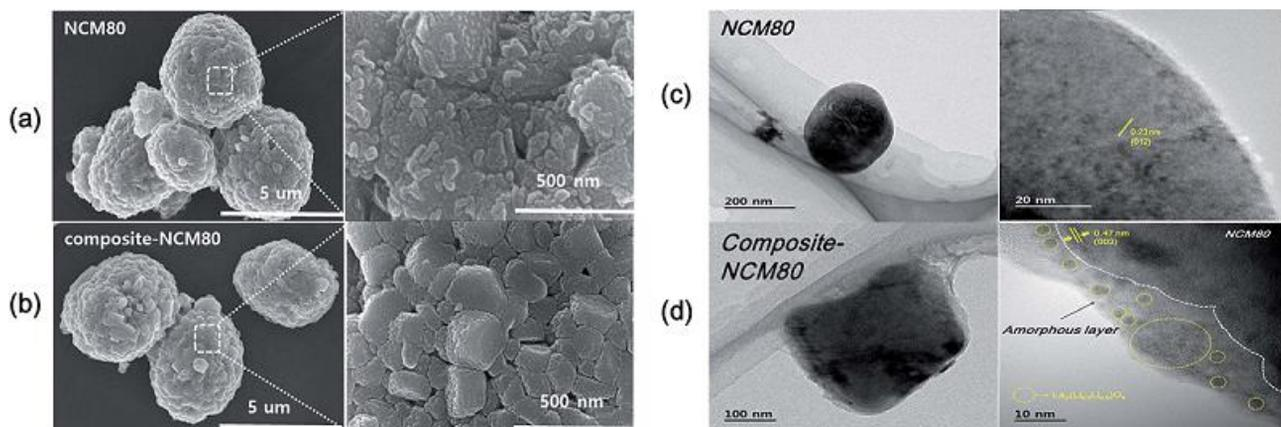
SEM images of (a) NCM80 and (b) composite NCM-LZAOH, and TEM images of (c) NCM80 and (d) composite NCM-LZAOH battery materials synthesized in Taylor Crystallizer
