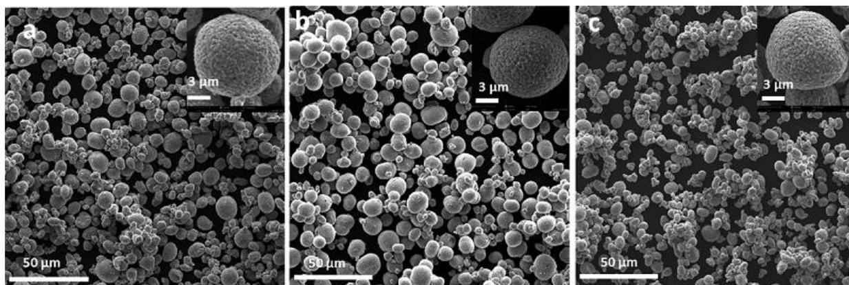
SEM images of (a) LNO, (b) LNMO, and (c) LNCO powder materials co-precipitated in Taylor Vortex Reactor (TVR) at MERF, Argonne National Laboratory
