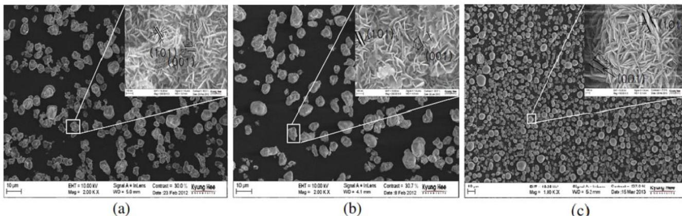
Morphology of NMC Hydroxide Produced in Couette-Taylor Crystallizer at (a) 700rpm 15min (b) 700rpm 30min (c) 1500rpm 30min
