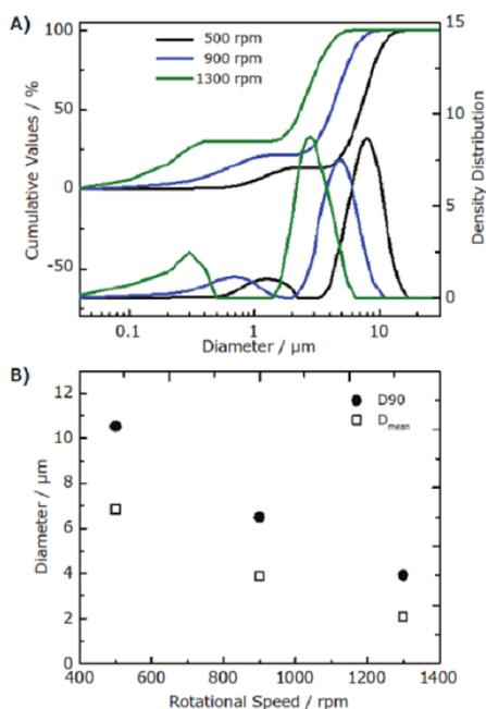
(A) NMC811 cumulative values and density distribution produced by Taylor Vortex reactor. (B) Average D90 values and PSD of Taylor-made NMC battery materials
