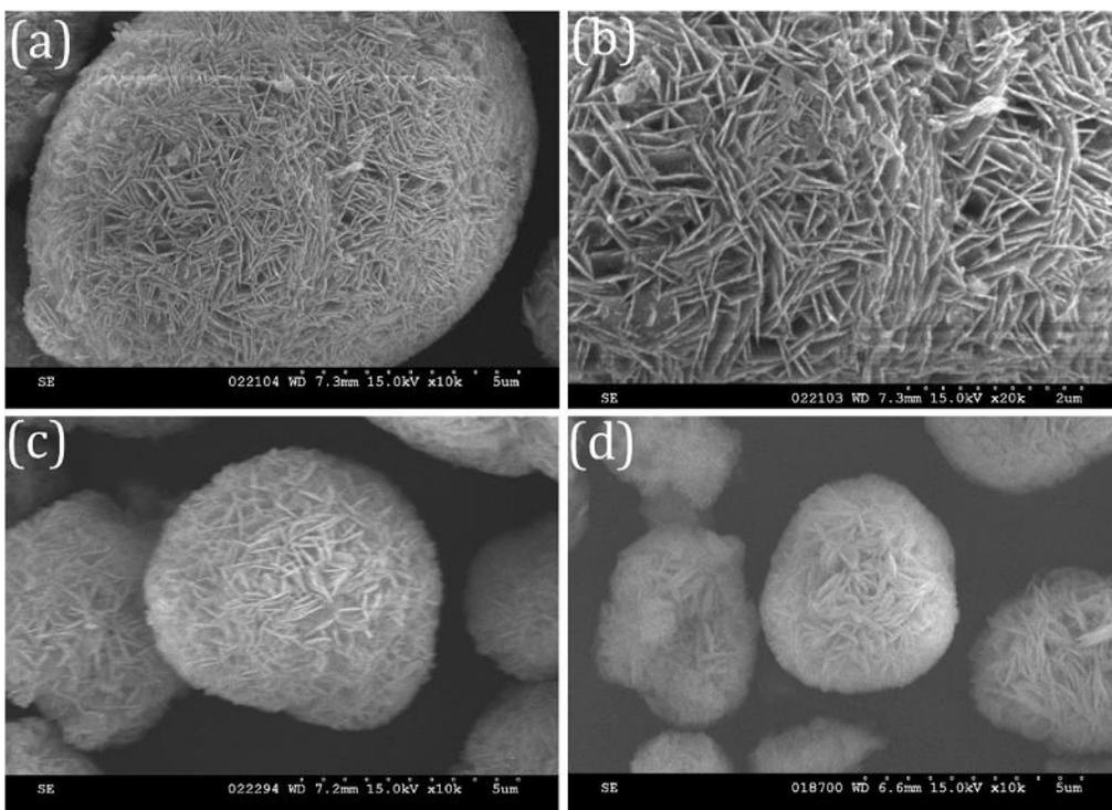
(a) SEM images of NCA Hydroxide materials prepared by Couette-Taylor Crystallizer at (a, b) 600 rpm, (c) 900 rpm, and (d) 1200 rpm.
