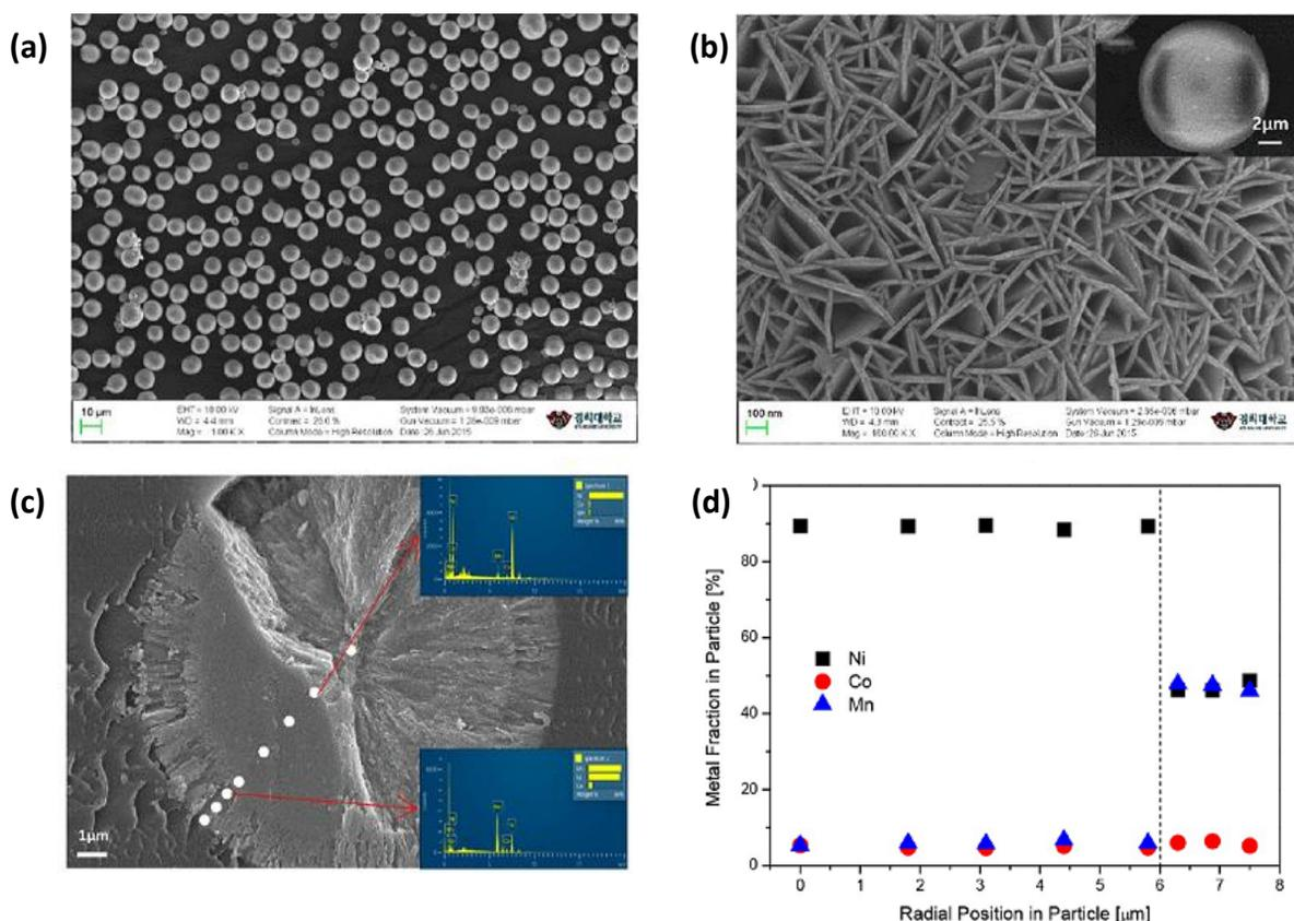
Morphology of (a) core particle shape, (b) surface of core particle. (c) EDS cross-sectional image of 1-2  $\mu\text{m}$  thick shell layer (c) experimental metal compositions of core and shell reflect theoretical values.
