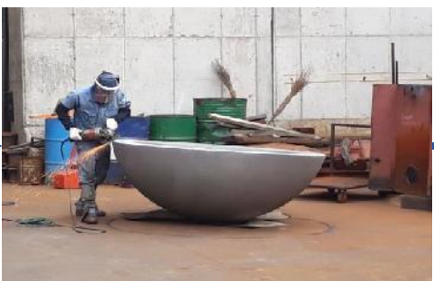
Edge Preparation using Turntable
