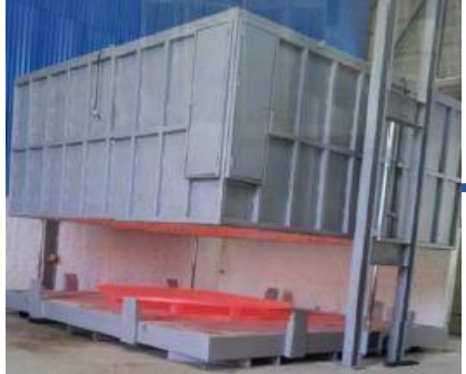
Plate Heating using Electric Furnace
