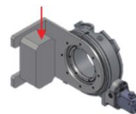
② Unbalance load torque due to gravity.
